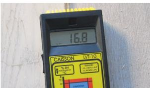
The relative humidity must lie between 40-70%. If the relative humidity is too low, a humidifier must be used. If the humidity is too high, a dehumidifier must be used.
